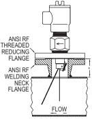
Flange Installation \*Flange face to pipe O.D. specified by customer. Normally should not exceed 5" (172)
