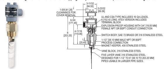
The Series V4 Flotect® Vane Operated Flow Switch is rugged and reliable, ideal for automatically protecting equipment and pipeline systems against damage from reduction or loss of flow. Time tested in thousands of pipeline installations and processing plants around the world this Series is Weatherproof, designed to meet NEMA 4 and Explosion-proof (listing included in specifications). This series can be used in pipes 1-1/2" (38.10 mm) and up.
